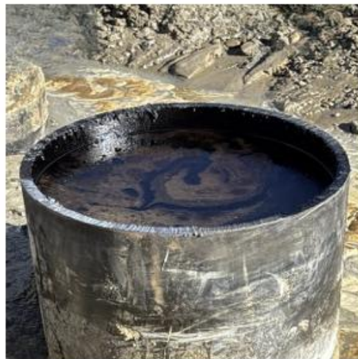
An after excess casing is removed. Oil emulsion observed inside the 24-inch casing.
