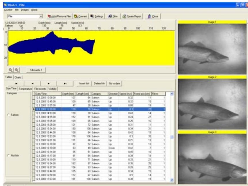
**Figure 5.** The Vaki Riverwatcher can be supplied with a digital camera system to record video or still images of fish passing through the scanner. The scanner triggers the camera to capture between 1 and 5 digital photos or a short video clip of each fish. The computer
