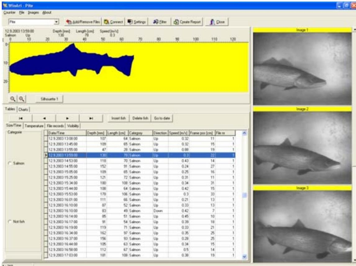
Figure 6. The Riverwatcher can be supplied with a digital camera system to record video or still images of fish passing through the scanner. The scanner triggers the camera to capture between 1 and 5 digital photos or a short video clip of each fish. The computer then automatically links the digital images to the other information contained in the database for that individual fish such as size, passing hour, speed, silhouette image, temperature etc. Image taken from Vaki, Inc. website:
