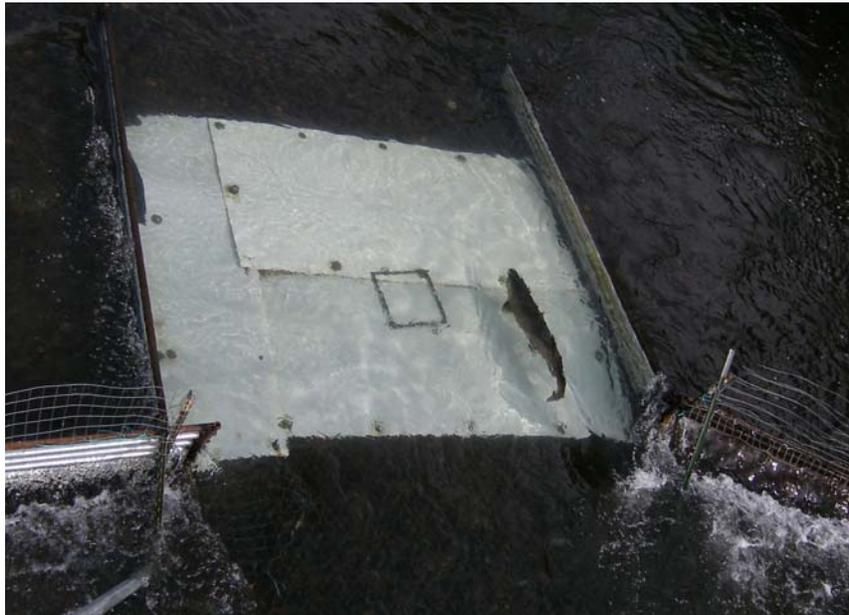
**Figure 8.** An example of favorable conditions for optical video cameras. The image shows a fall-run adult Chinook salmon (approximately 91 cm in length) passing the Battle Creek weir. Photo credit: Doug Killam, CDFG.
