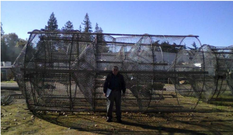
**Figure 4.** A large wire fyke trap constructed by CDFG Region 3 for striped bass population assessments. Traps are composed of chain link fencing, steel hoops, wooden stringers, and plastic mesh (in fish pot only).
