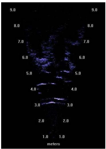
Figure 11. DIDSON image of migrating sockeye salmon with the salmon images outlined. The remaining signal comes from a combination of river bottom and volume reverberation, Wood River, July 2, 2002. Image was taken from Maxell and Gove (2004)
