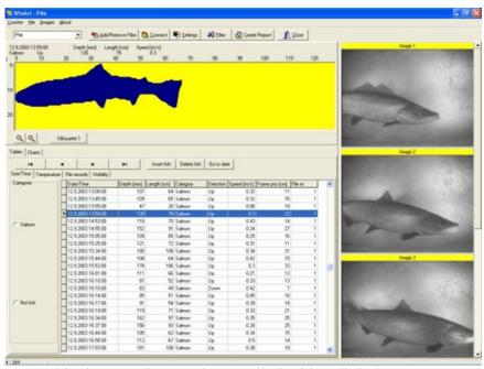
**Figure 5**. The Vaki Riverwatcher can be supplied with a digital camera system to record video or still images of fish passing through the scanner. The scanner triggers the camera to capture between 1 and 5 digital photos or a short video clip of each fish. The computer
