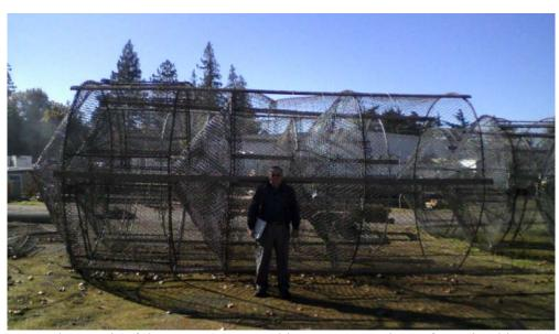
**Figure 4**. A large wire fyke trap constructed by CDFG Region 3 for striped bass population assessments. Traps are composed of chain link fencing, steel hoops, wooden stringers, and plastic mesh (in fish pot only).
