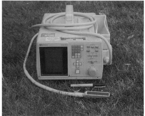
The veterinary ultrasound equipment used during this project is highly portable and may be readily transported and operated in the field. This photo depicts a 5 MHz transducer that is used for measuring fat and muscle thickness. Photo by Tom Stephenson.
