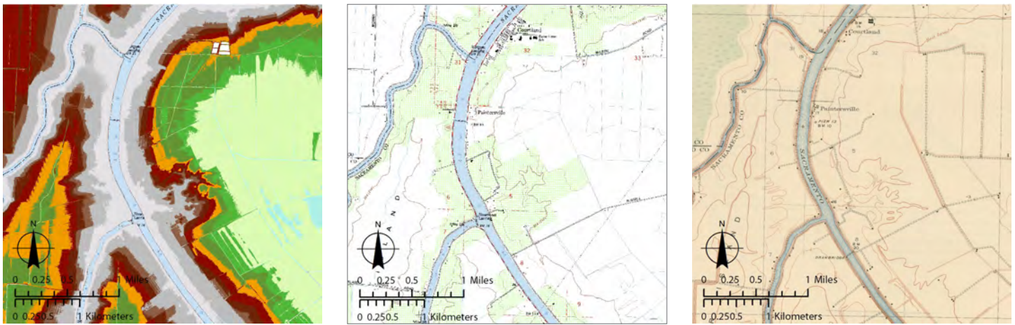
Figure 5. Natural river levees past and present. These images show the presence of elevated fluvial deposits along the Sacramento River revealed by the topography shown in the 1916 USGS topographic quad (left) and similar patterns today, as exemplified by the orchards depicted in contemporary USGS topographic quads (center) and elevations in LIDAR imagery (right). Because of their mineral sediments, these features have been relatively unaffected by subsidence. Potential riparian functions have shifted, and will continue to shift, upstream or downstream in response to changes in land use, sea level, and inundation frequency.
