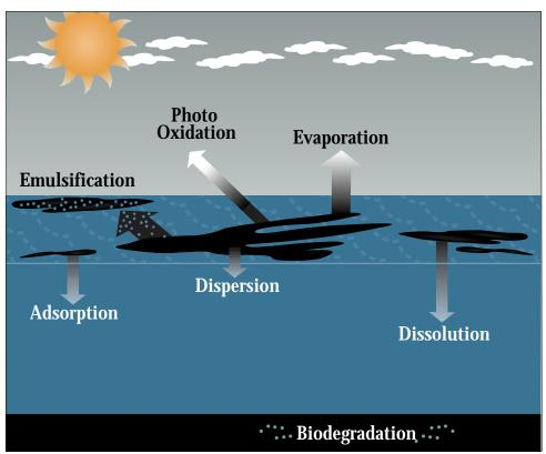
Emulsification is generally the primary weathering process of concern with spilled crude blends. Many crude blends emulsify quickly when spilled, creating a stable mousse that causes a persistent cleanup and removal challenge.
