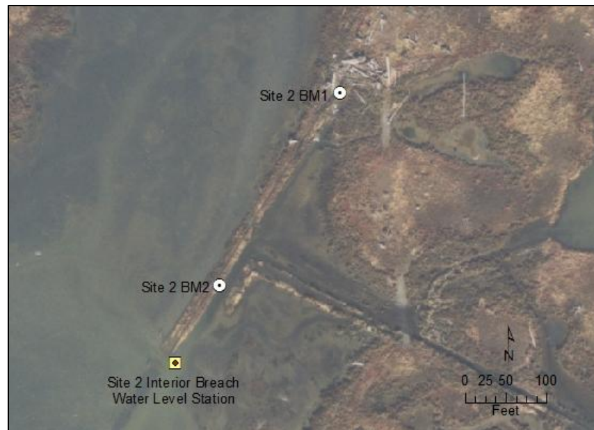
Figure 3-3. Site 2 Interior Breach plan view.
