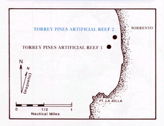
Center Coordinates Compass Bearing Year Constructed Materials Used Comments 32° 53' 35" N x 117° 15' 35" W Depth 44 ft. (MLLW) 359° (mag), 3 N miles from Point La Jolla Tower 1975, (augmented 1979) Area 1 acre (approx.) 3,000 tons quarry rock, augmented by concrete dock floats. This reef holds significant numbers of blacksmith, sheephead, and kelp bass. Few barred sandbass have been seen.
