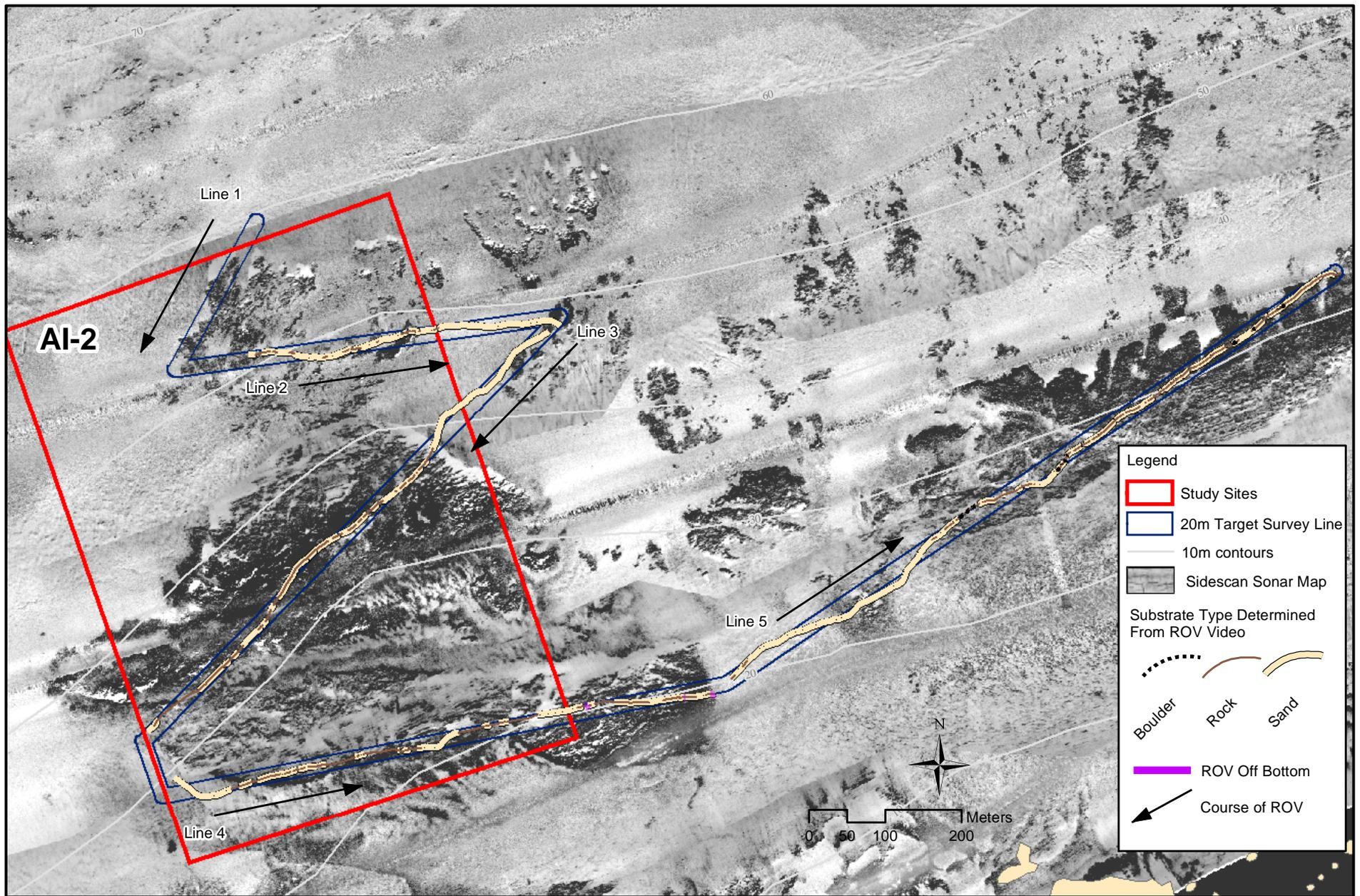
Figure 5. Habitats observed during a dive off Anacapa Island SMR site AI 2 on May 14, 2004 over shaded relief side scan sonar map. Planned  $\pm 10$  m navigational boundary in relation to smoothed ROV track line is color coded by observed habitat type of rock, sand, and boulder.
