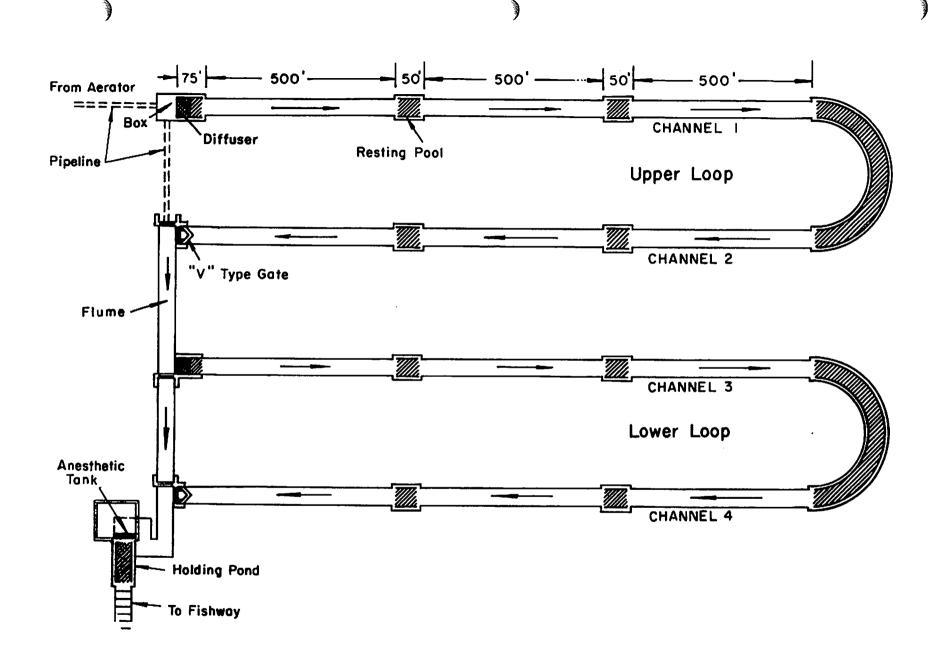
Figure 2. Diagram of the Makeluane River Spawning Channel
