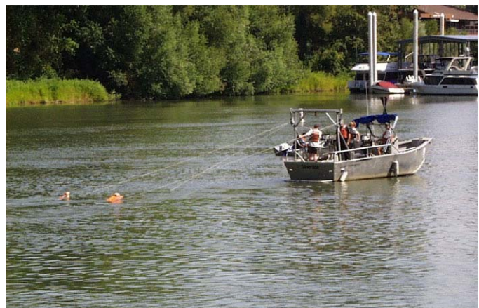
Photo 10 Sacramento and Mossdale Trawls: Midwater trawl being retrieved by Sacramento Trawl Survey crew on the Research Vessel Silverside.
