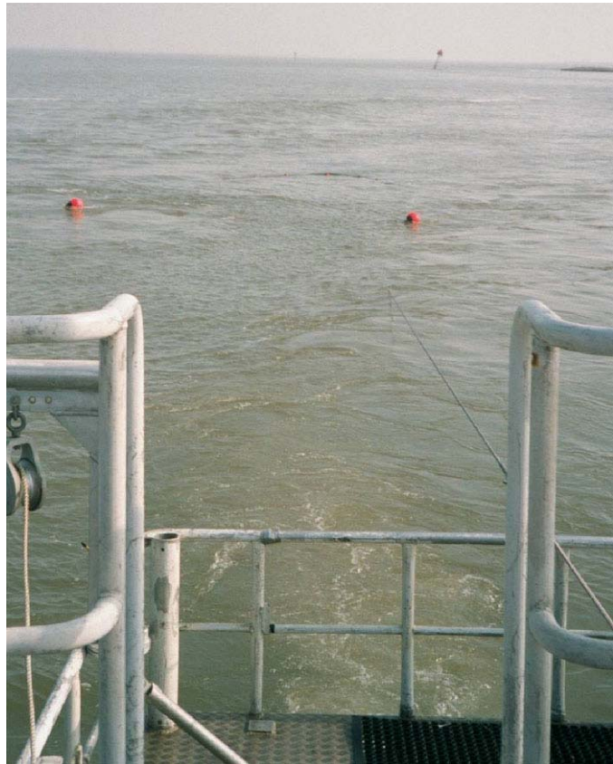
Photo 6 Spring Kodiak Trawl. Kodiak trawl underway looking astern from Research Vessel Scrutiny flying bridge; orange floats mark the net end. The second boat is out of view to the left.
