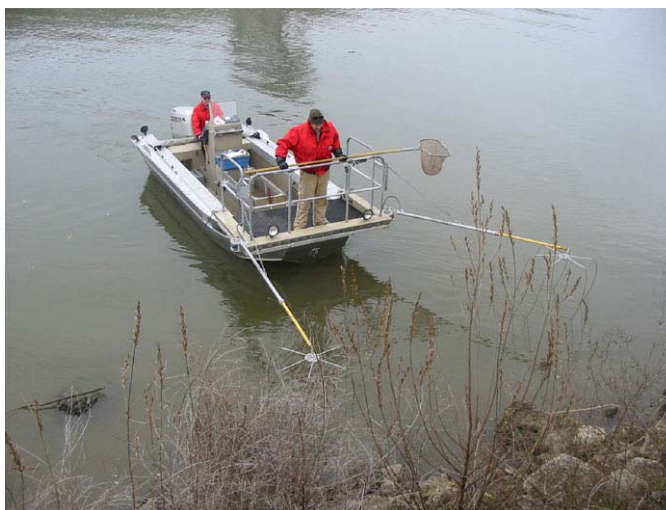
Photo 7 Resident Fishes Survey. Fish within a created electrical field are attracted to boat's forward-mounted anode probes.
