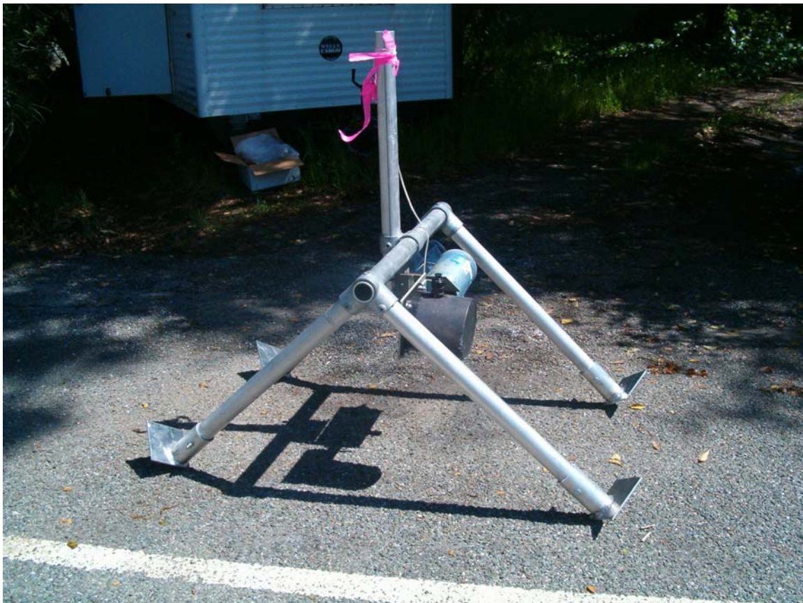
Figure 4. Photograph of aluminum frame mount used to deploy the split beam transducer in Mill Creek in 2006. The transducer and dual-axis rotator are shown mounted on the frame. An identical frame was used to deploy the DIDSON.
