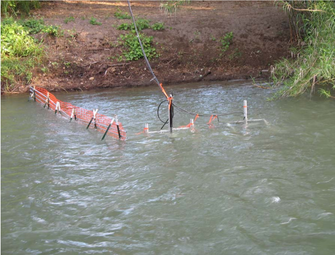
Figure 5. Photograph showing the fish fence and deployment of the split beam transducer and DIDSON off the river right bank at the Sherwood Bridge study site on Mill Creek in 2006.
