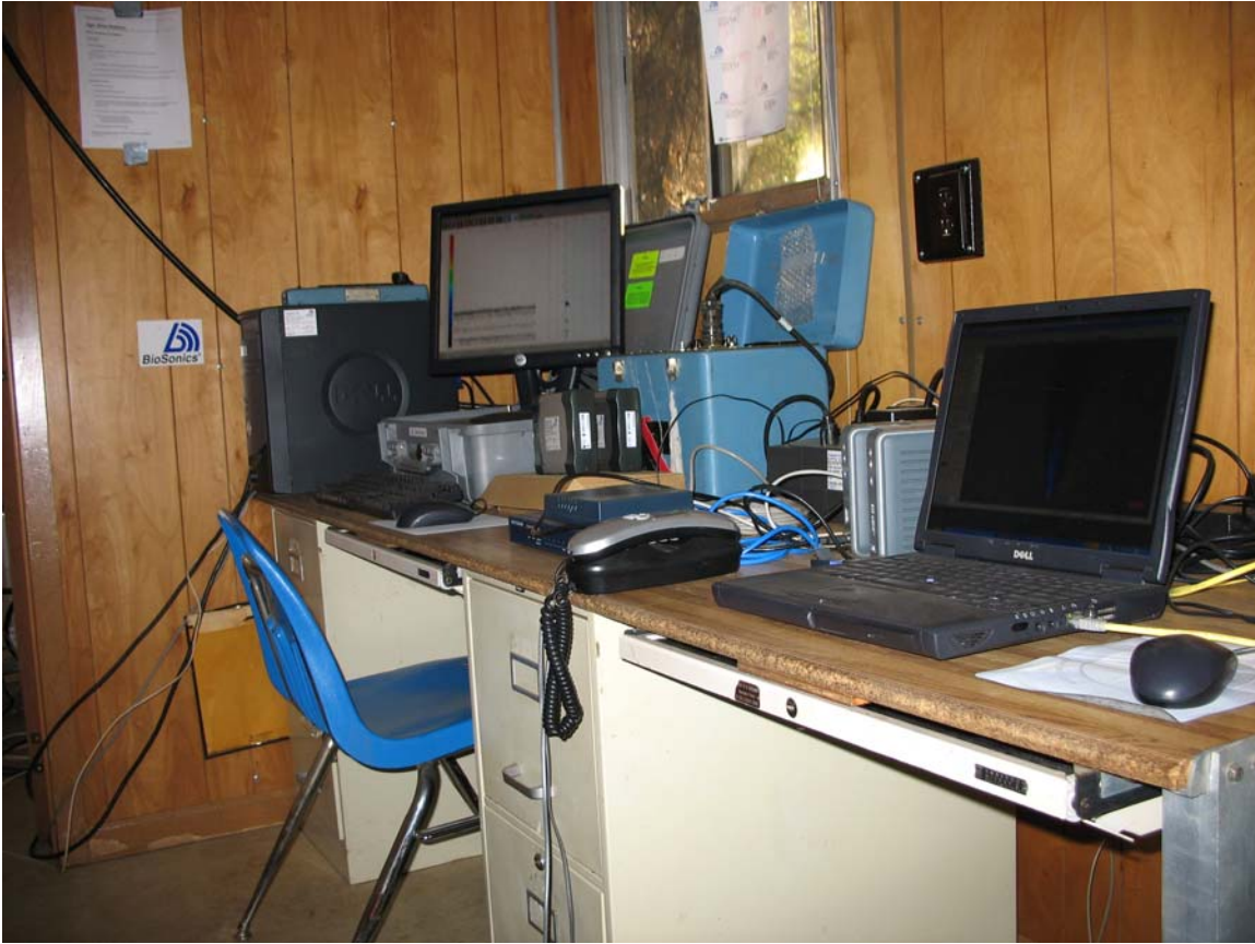
Figure 10. Split-beam echo sounder surface unit, data collection PC, rotator control box, and data collection PC installed in project trailer. Laptop on the right controlled the DIDSON system.
