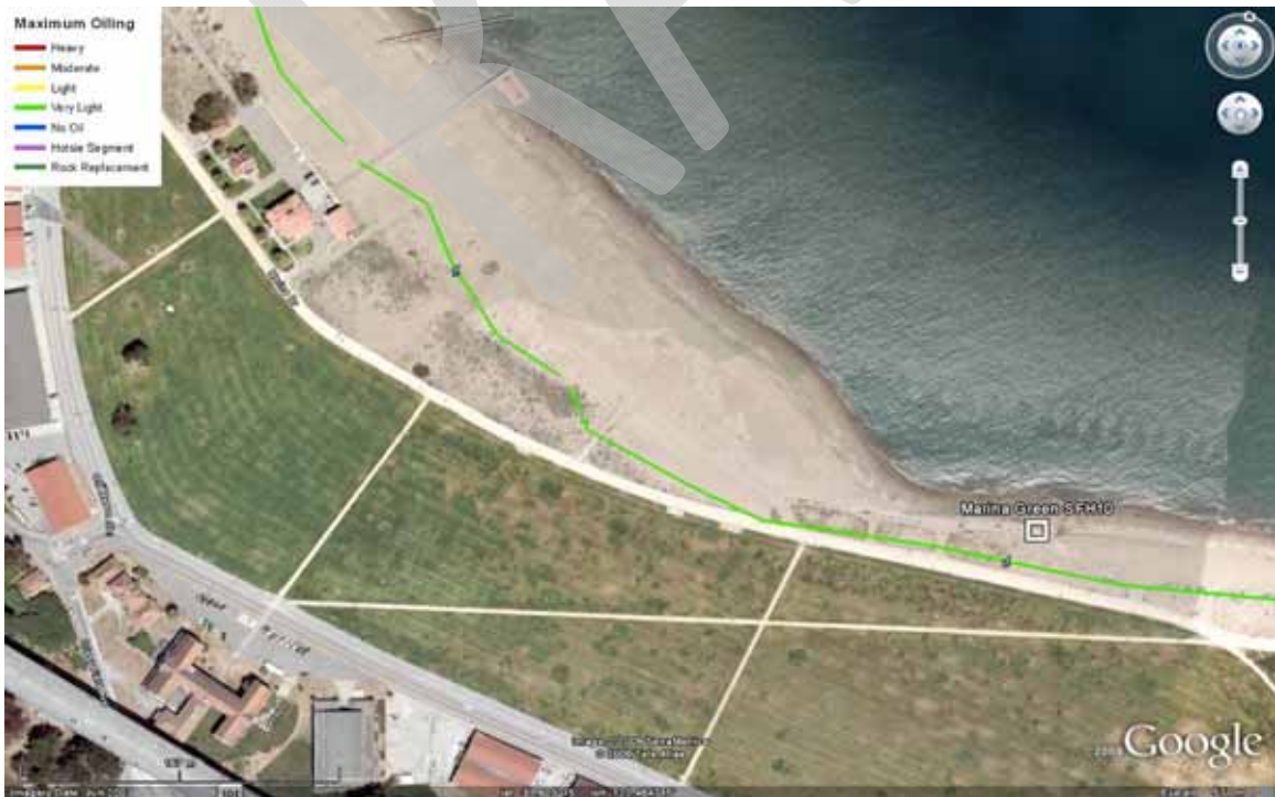
Figure 1-11: The site sampled at Marina Green SFH10 showing the level of oiling.
