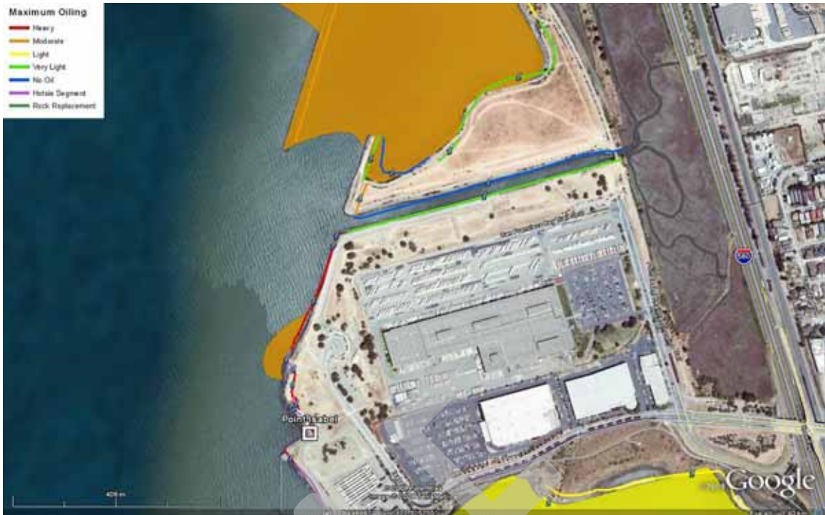
Figure 1-14: The site sampled at Point Isabel showing the level of oiling and the Hotsie segment. The Hotsie segment is the area where power washing took place.
