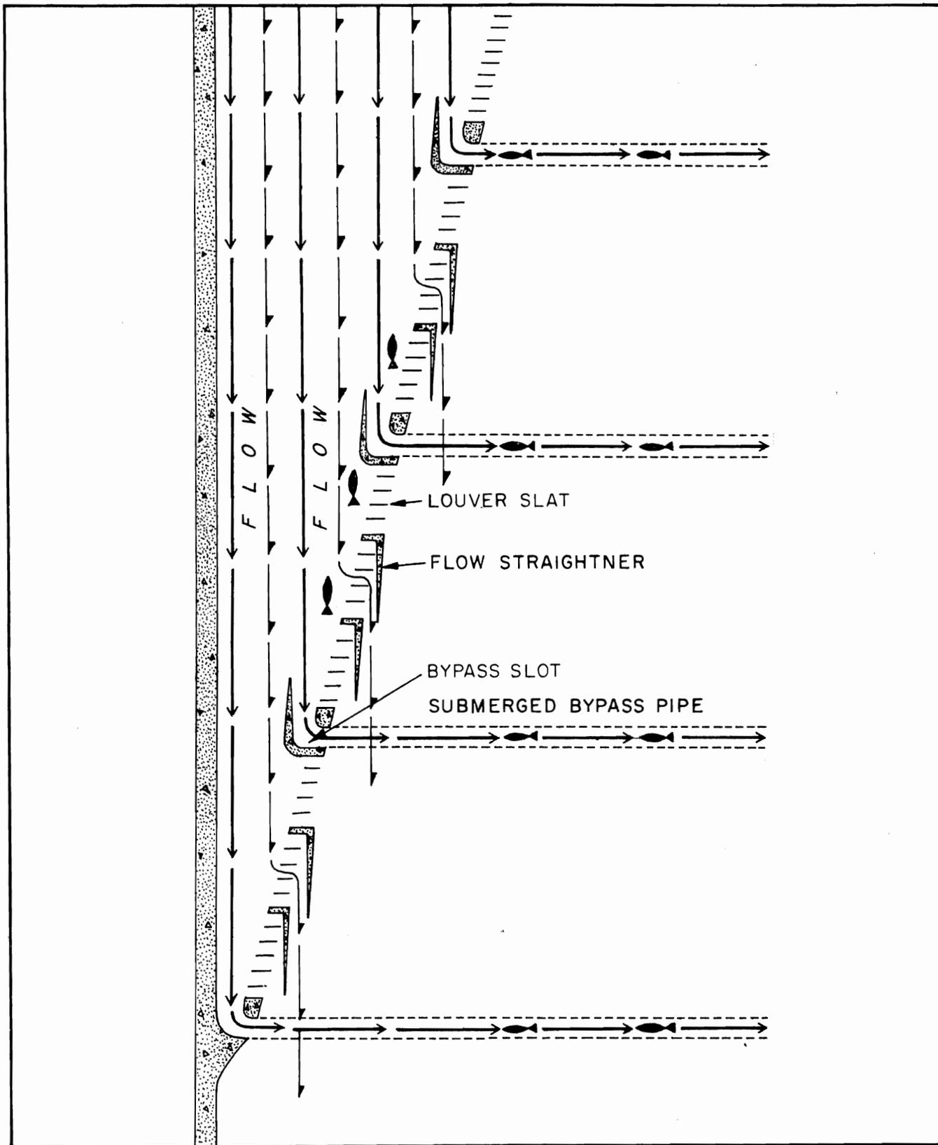
Figure 1. Diagram of a Louver System.
