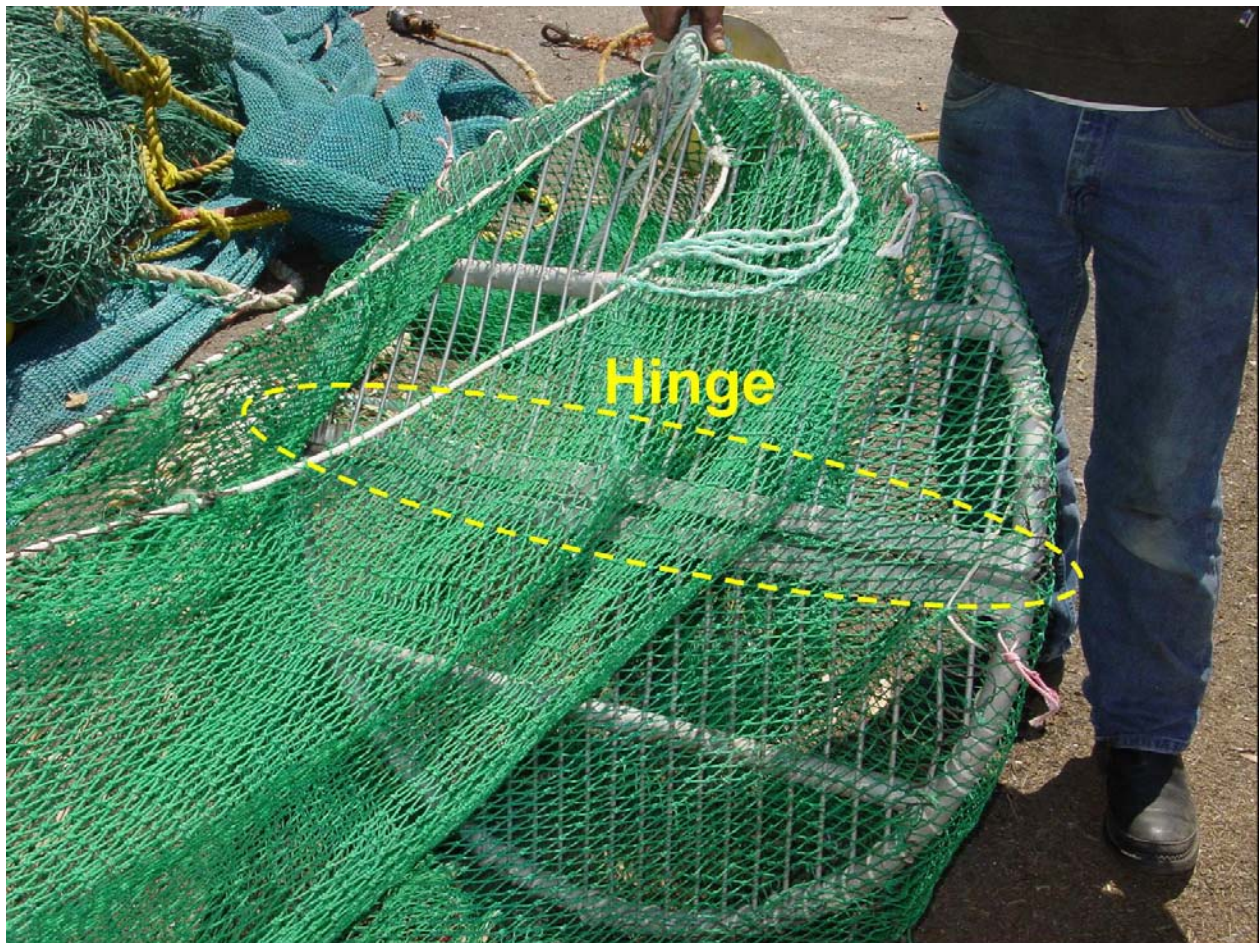
Figure 4. Photograph of a hinged, or folded, rigid-grate BRD. Photo credit: A. Frimodig, CDFG.
