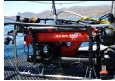
DFG regularly uses “BOB” (a remotely operated vehicle) to survey MPA’s in the northern Channel Islands.
