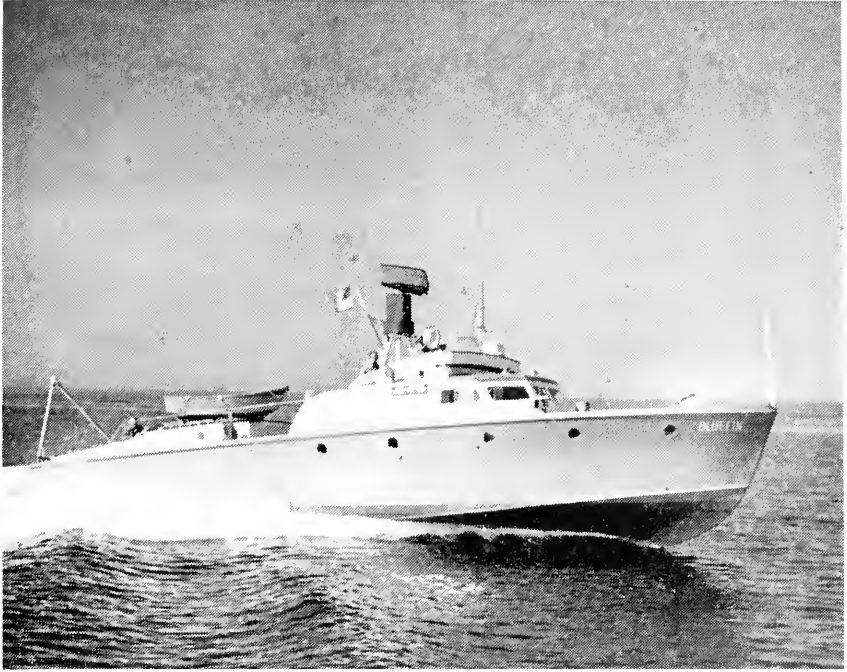
FIGURE 20. 63-foot Fish and Game patrol boat BLUEFIN. The commission operates two of these vessels in Southern California waters. Equipped with two 630-h.p. Hall Scott Defender engines, radar, radio and full marine equipment. Photograph by Vernon M. Hadon, San Pedro.
