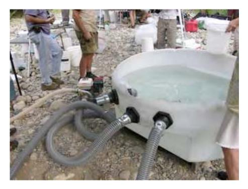
And for those unfamiliar with suction dredging the following photograph will reveal that the dredge floats on the water and is intended to vacuum the overburden from the river or creek bottom. The vacuumed material, (i.e., clay, sand, rocks,) pass through a sluice box that captures the heavy materials (i.e., gold, lead, platinum, mercury) while returning the other materials back to the receiving water.
