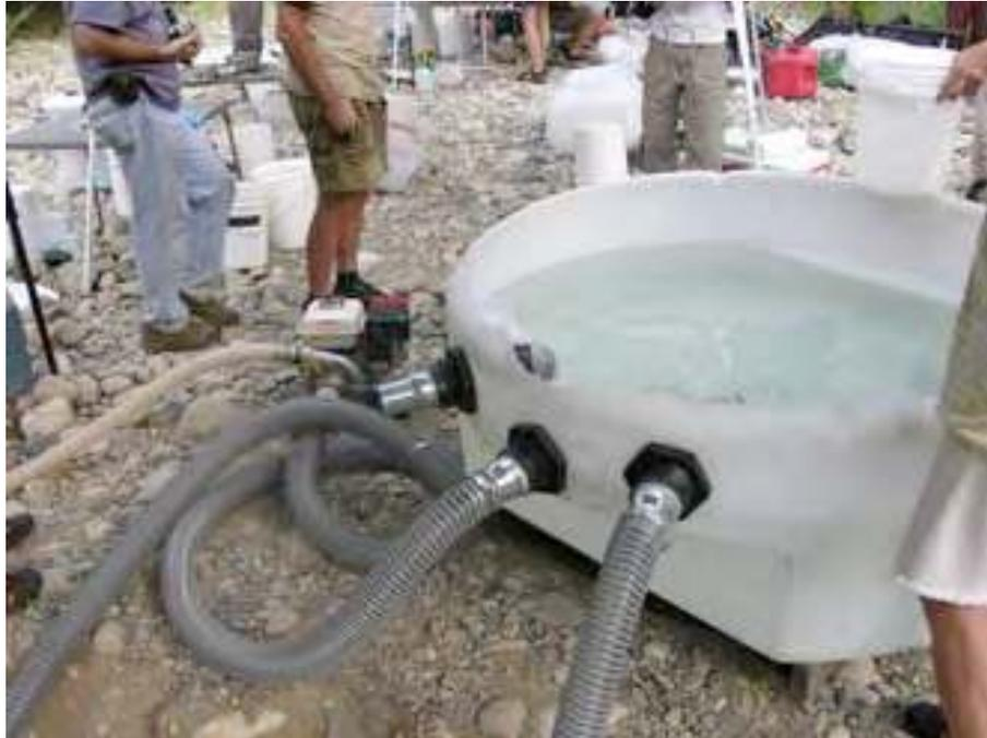
And for those unfamiliar with suction dredging the following photograph will reveal that the dredge floats on the water and is intended to vacuum the overburden from the river or creek bottom. The vacuumed material, (i.e., clay, sand, rocks,) pass through a sluice box that captures the heavy materials (i.e., gold, lead, platinum, mercury) while returning the other materials back to the receiving water.
