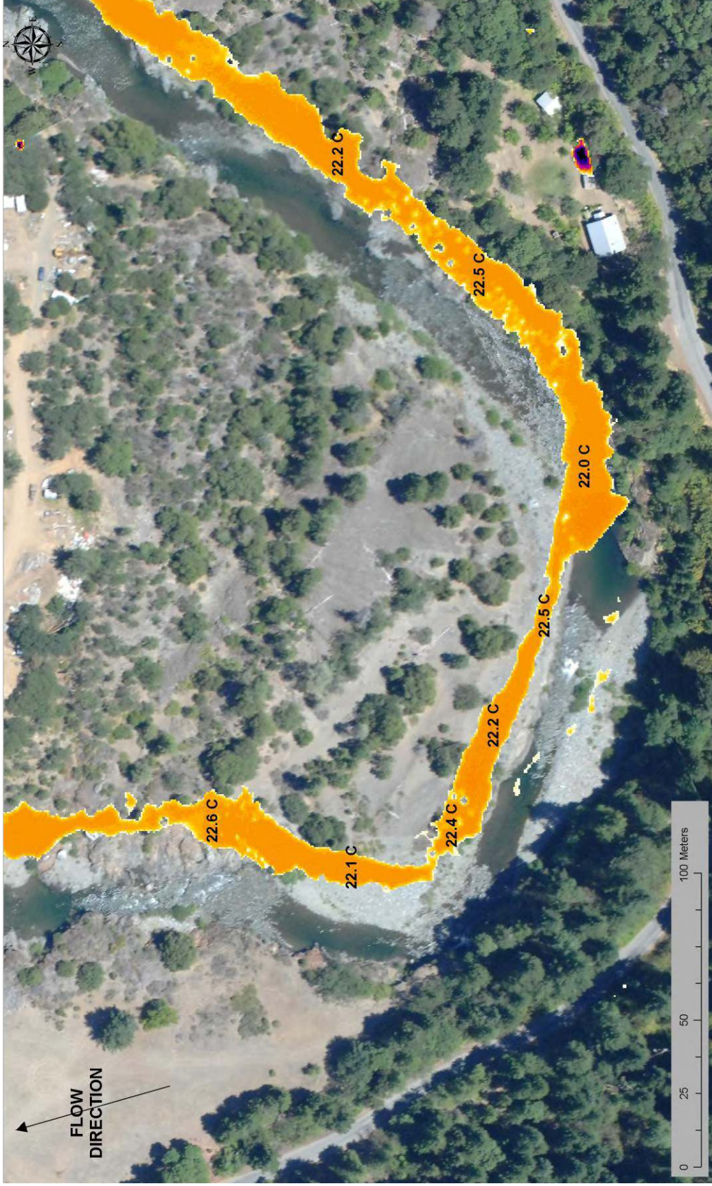
South Fork Image 2 – The TIR/true color image pair at river mile 0.58 shows the type of variability seen in pool/riffle sequences.. The images are offset in order to show the location of the pools and riffles in the true color imagery.
