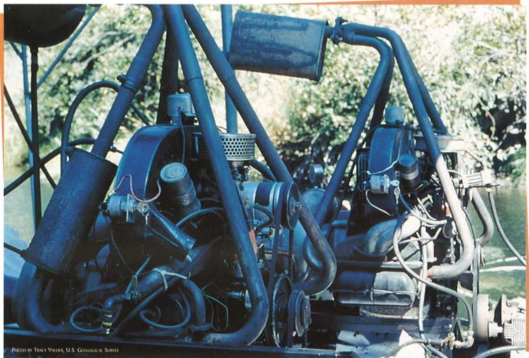
Suction dredge engines outfitted with mufflers.
