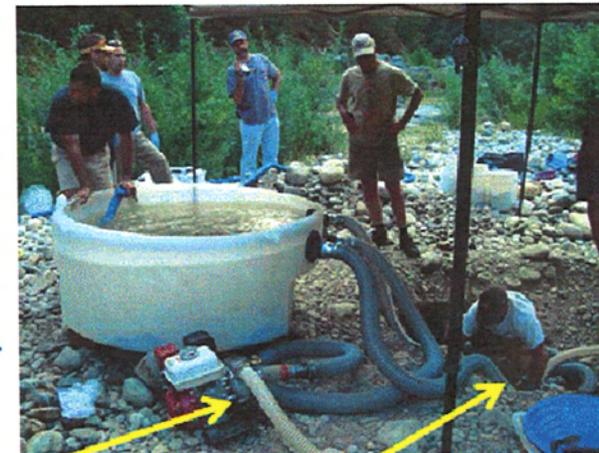
Hg and silt forced through pump impeller resulting in fragmentation of mercury into finer and finer particles
