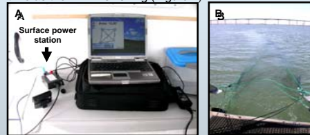
Figure 3. Net Track A) real time display of net mouth area during tow and B) responder configuration in the MWT net at end of tow.
