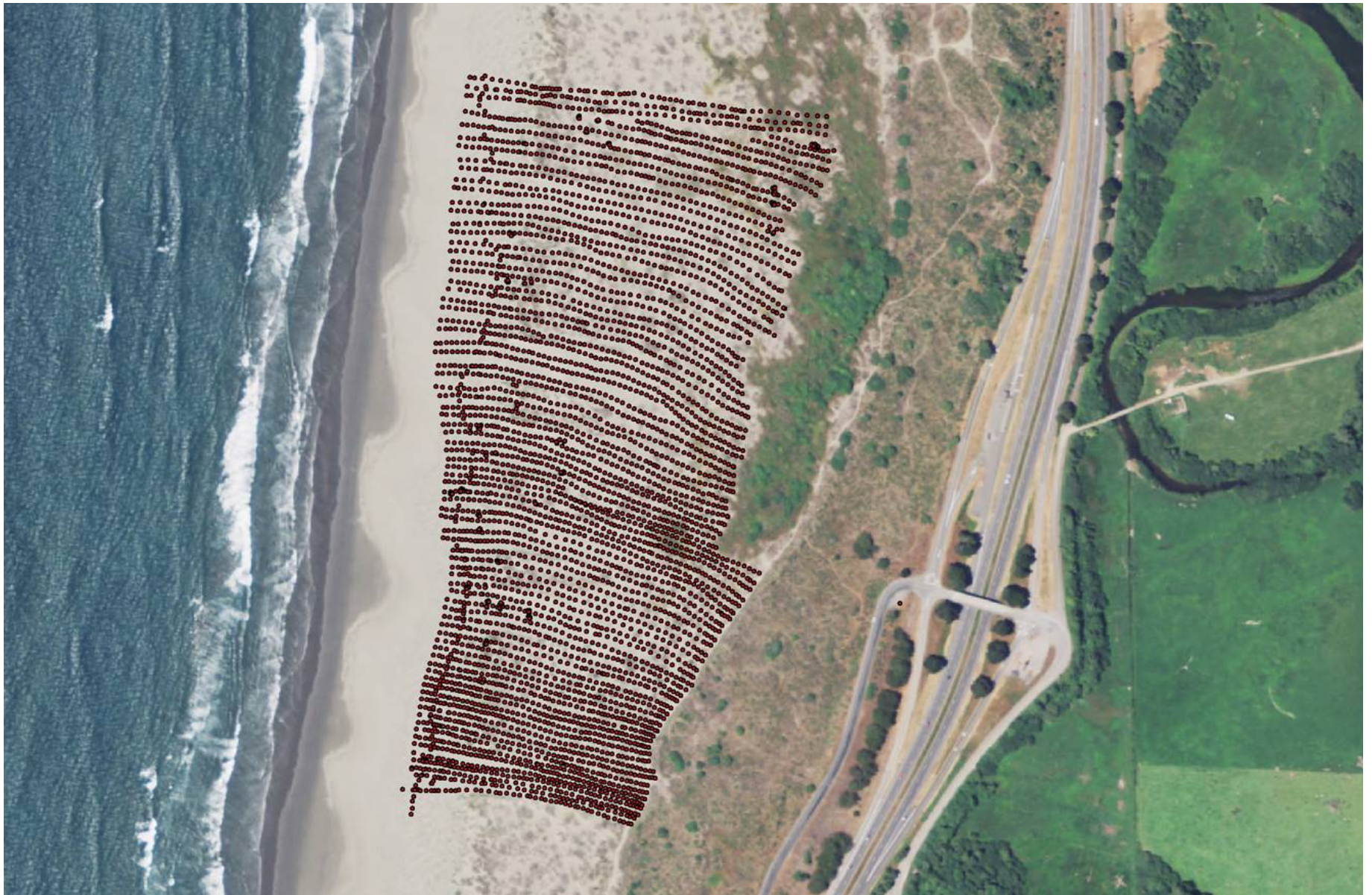
Figure 2.0 Dune morphology data points taken by the RTK 1 year after initial treatment.
