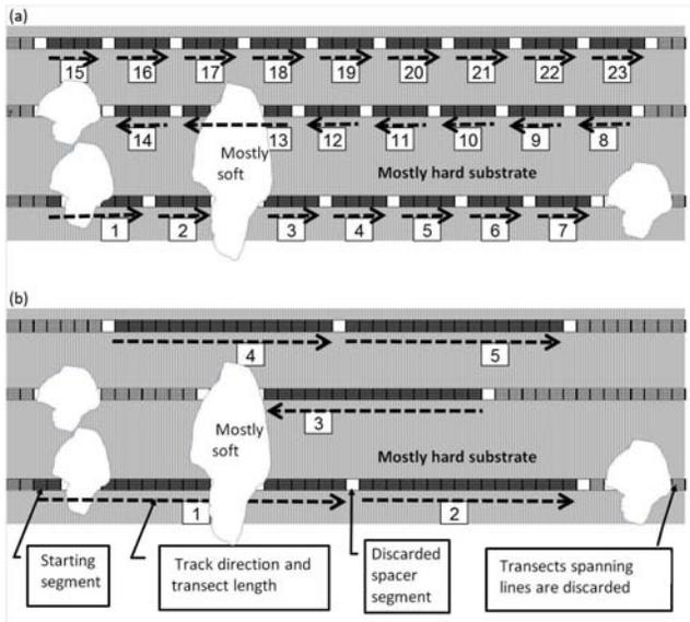
Figure 3. Illustration of how (a) twenty-three 100 m<sup>2</sup> and (b) five 400 m<sup>2</sup> transects were created using (a) four and (b) sixteen 25 m<sup>2</sup> segments respectively. Shown are the same three track lines at the start of a hypothetical study area.
