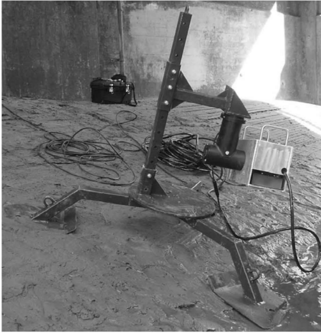
Figure 1. DIDSON mount design used for our trial on the San Lorenzo River, California in March 2006. Photograph by authors.
