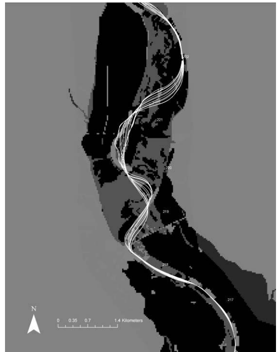
Woodson Bridge Shasta flow with the revetment at RM 220-222 (Right bank) at Kopta Slough removed.
