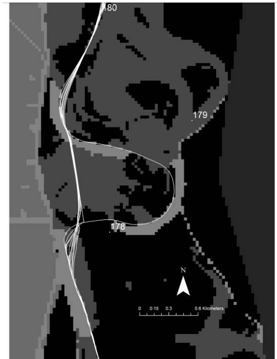
Ord Ferry Shasta flow with the revetment at RM 179 (Right bank) at the Llano Seco Riparian Sanctuary removed.
