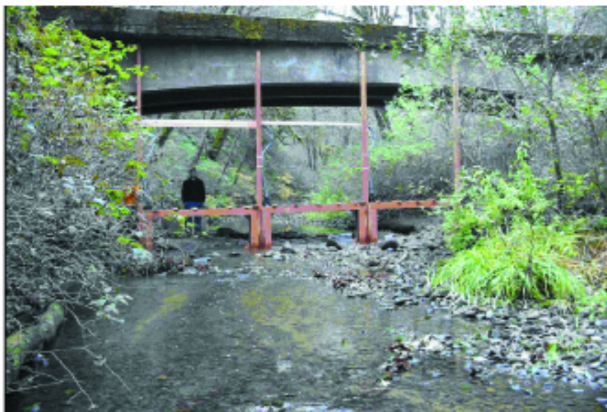
Figure 4. Example of structure for PIT tag detection antenna.
