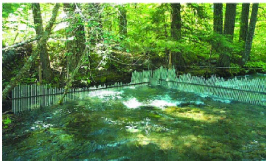
Figure 5. Alaska-style weir with Vaki fish detector, McKenzie River, Oregon.
