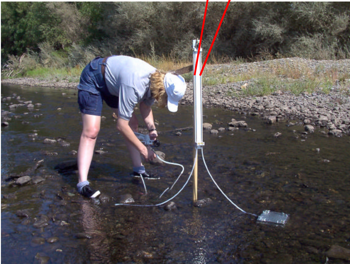
Figure 9: A manometer board is attached to subsurface sampling tubes to measure differences in hydraulic head. Higher head in the stream indicates losing conditions, although gaining conditions (upwelling) are common at the downstream ends of riffles and gravel bars. A baffle box is used to restrict current flow and minimize pressure differences past the open end of the tube.
