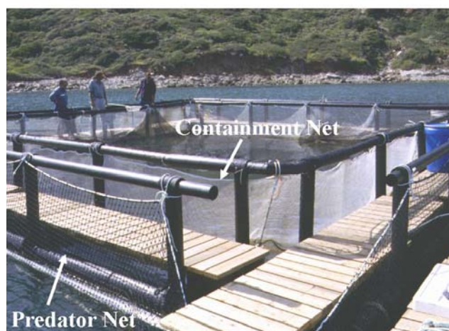
Figure 7. Example of placement of predator and containment nets.
