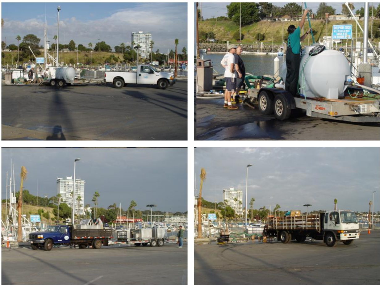
Figure 31. Photographs of various truck-hauling configurations used to transport juvenile white seabass. Photograph in lower left quadrant shows most commonly used configuration.
