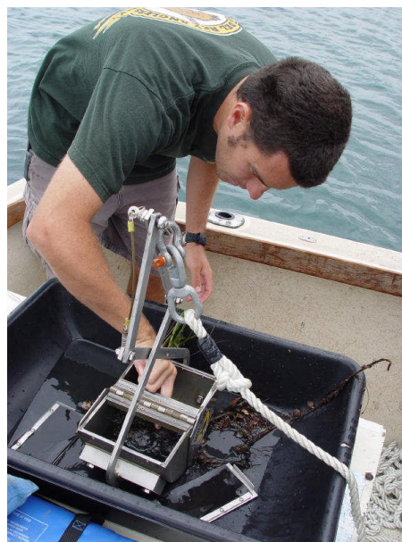
Figure 6. Technician removing debris from surface layer of sample collected using Petite Ponar grab.
