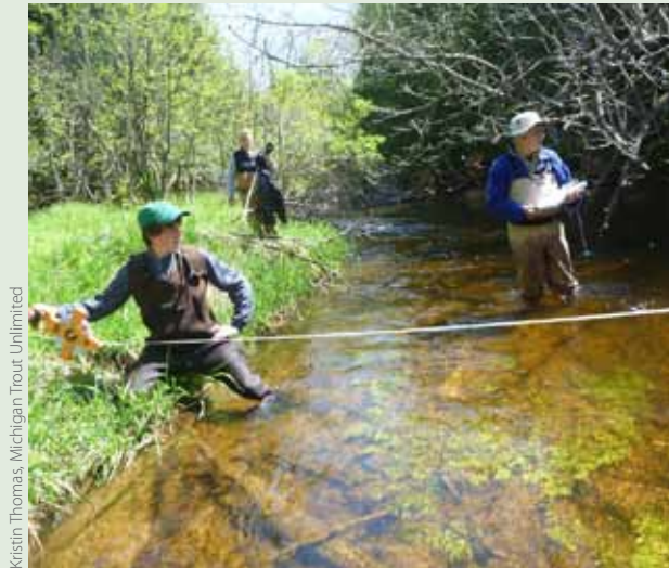
Measuring stream width along a small Michigan stream. Three or four people makes a good size team for habitat mapping.
