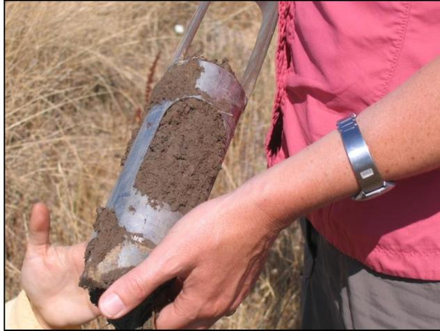
**Figure 3.1:** Open bucket auger used to extract soil samples.
