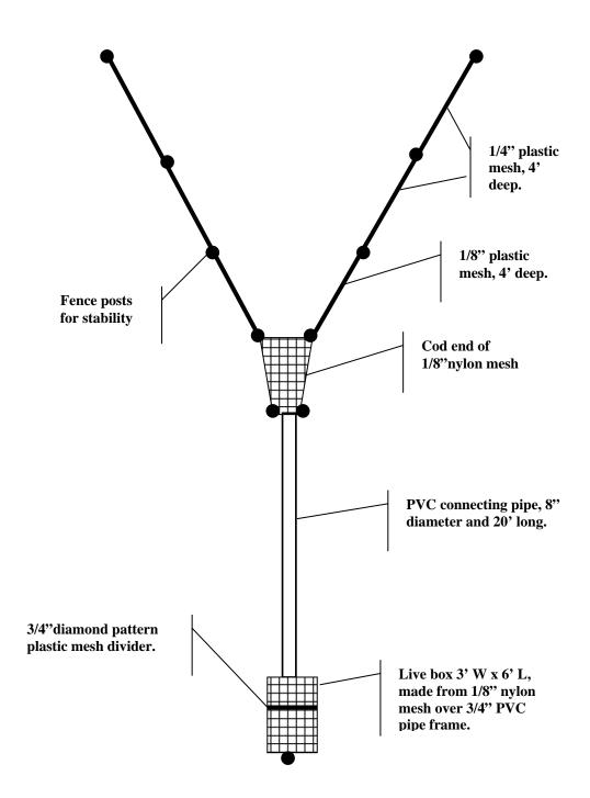
Figure 9. Diagram of fyke net smolt trap.
