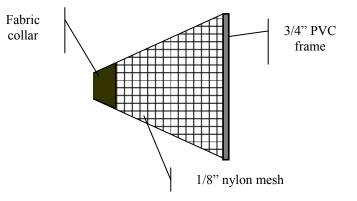
Figure 11. Diagram of fyke net cod-end.
