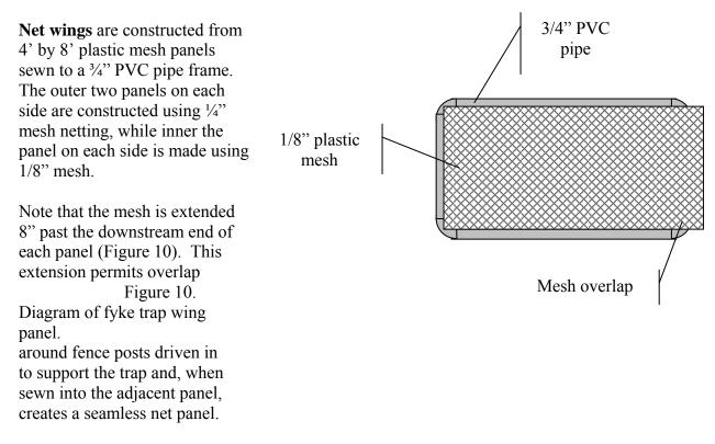
Net wings are supported by eight fence posts. One post is placed on the upstream end, one of the downstream end and one at each panel juncture. Mesh panels are then secured to fence posts using electrical ties. Sand bags filled with stream gravel are stacked along the inner and outer side of the lower mesh panel for further stability.
