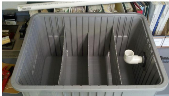
Figure 2. Interior view of biobox plates that provide suitable surfaces for mussel and mudsnail settlement.
