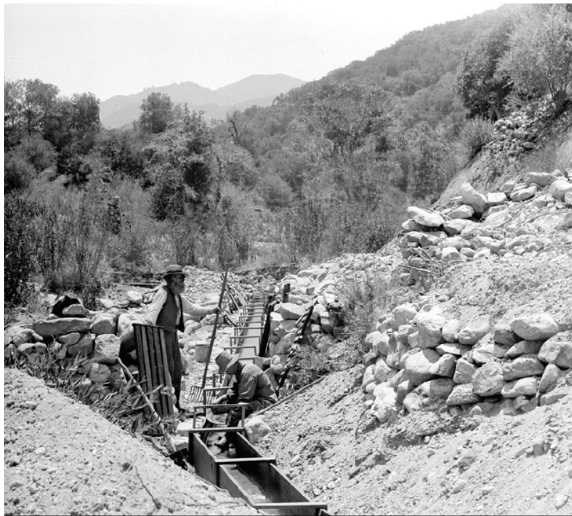
Figure 3. Gold mining sluice in Placerita Canyon, 1800s-1900s. (Image from a glass-plate negative by Frank Evans, Santa Clarita Valley History in Pictures www.scvhistory.com ; Harvey 2007).
