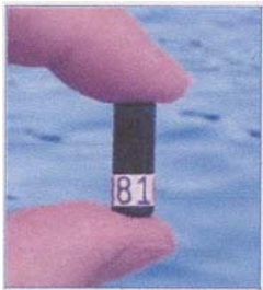
Fig. 5. Miniature coded ultrasonic beacon recently developed by Vemco, Ltd. of Halifax for tracking juvenile sturgeon and salmon smolts. This miniature tag has a diameter of 7 mm, minimum length of 17.5 mm, and a battery life of approximately 200 days.
