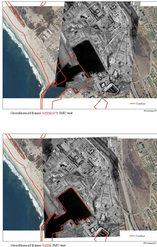
Figure 1. Auto-georeferenced imagery of San Diego coastline using only DGPS coordinate information (top) and using DGPS/IMU information (bottom).
