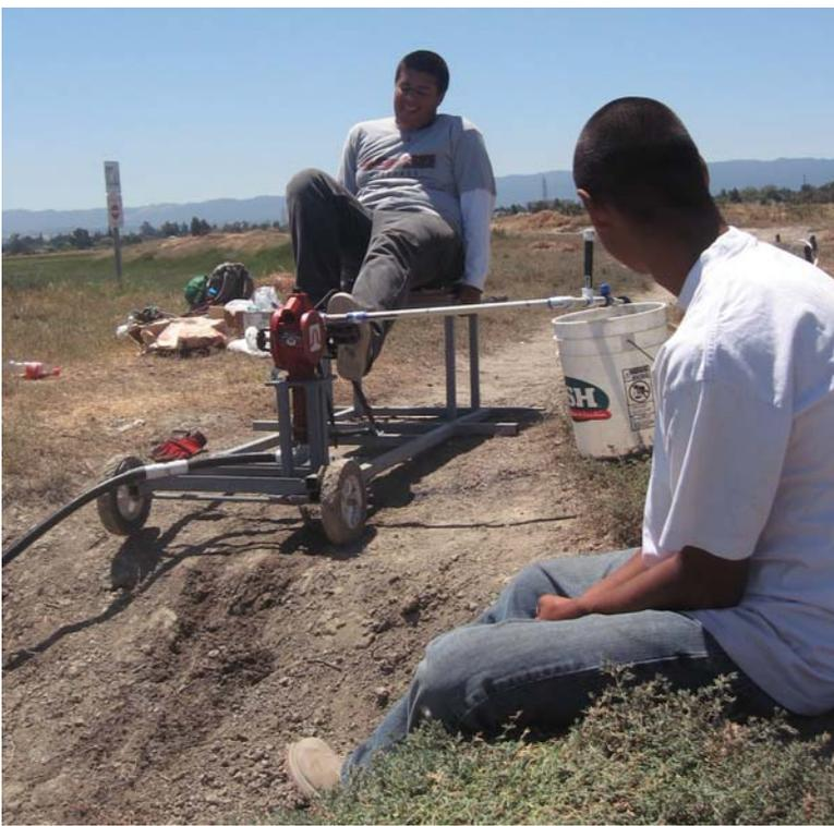
Pedal powered irrigation system for salinization.
