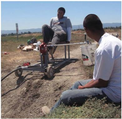
Pedal powered irrigation system for salinization.
