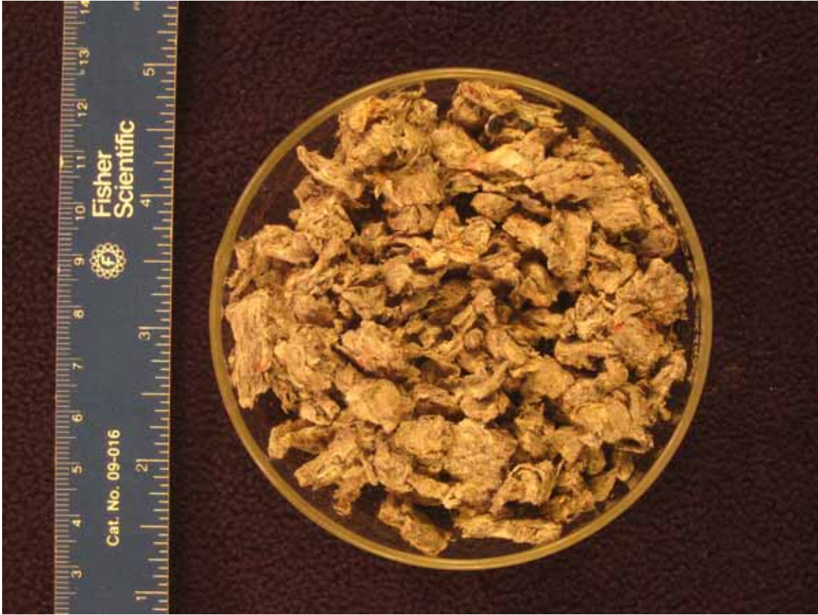
Photograph of dry CheetahSorb sample. Description: chunky, dry, shredded paper product and partially still identifiable material.
