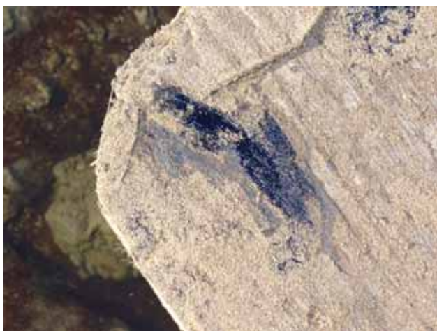
Fig. 11. Peat moss sorbent applied to wood plank after contaminated with oil spill tar. Rubbed with finger to exposed unabsorbed tar.
