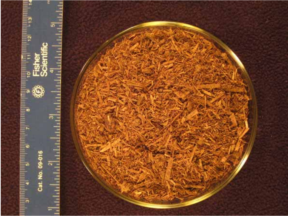
Photograph of dry NatureSorb sample. Description: dry, ground, fibrous, recycled cellulose material.
