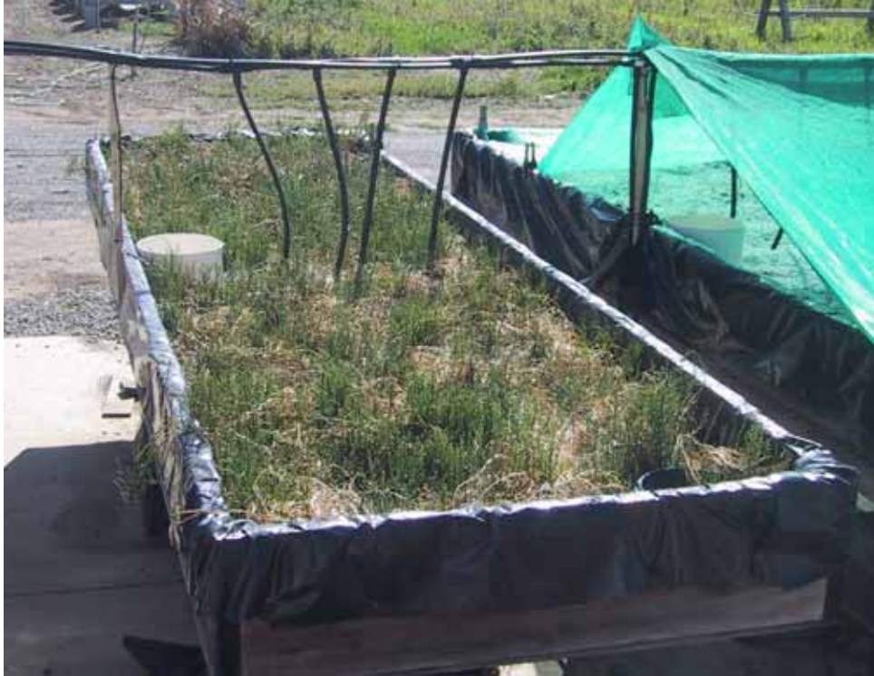
Fig. 1. Large vegetated tanks with overhead lines to supply air to subsurface aeration hoses from van pump, and water to float valves.
