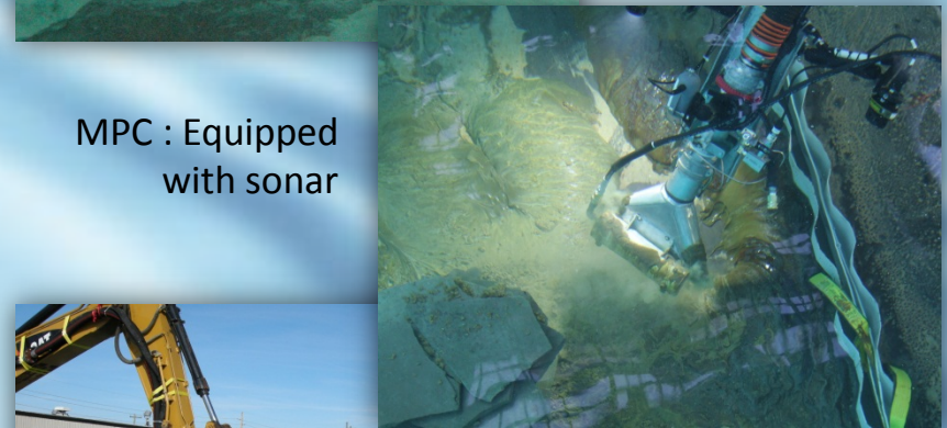
Oil Stop/AMPOL Sub-Dredge: Submersible dredge with underwater camera
