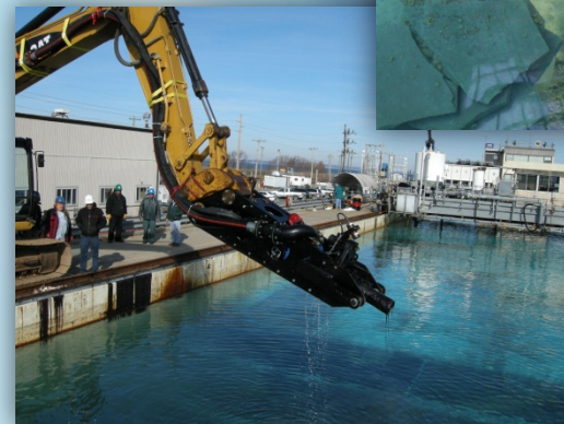
Oil Stop/AMPOL Sub-Dredge: Submersible dredge with underwater camera
