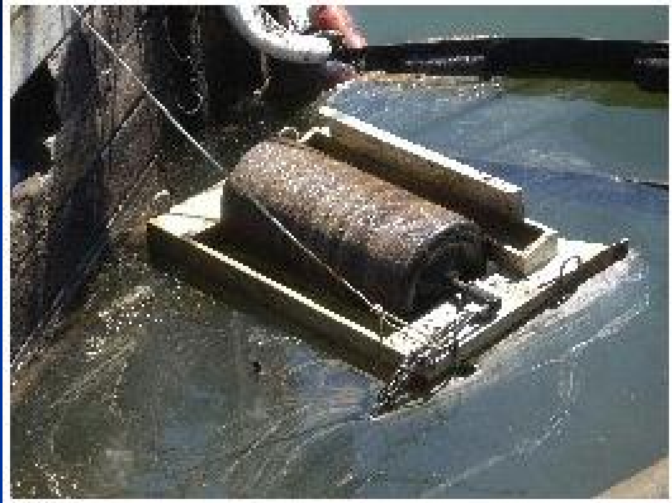
CLEAN HARBORS COOP – 36 INCH COATED DRUM SKIMMER ON SPILL
