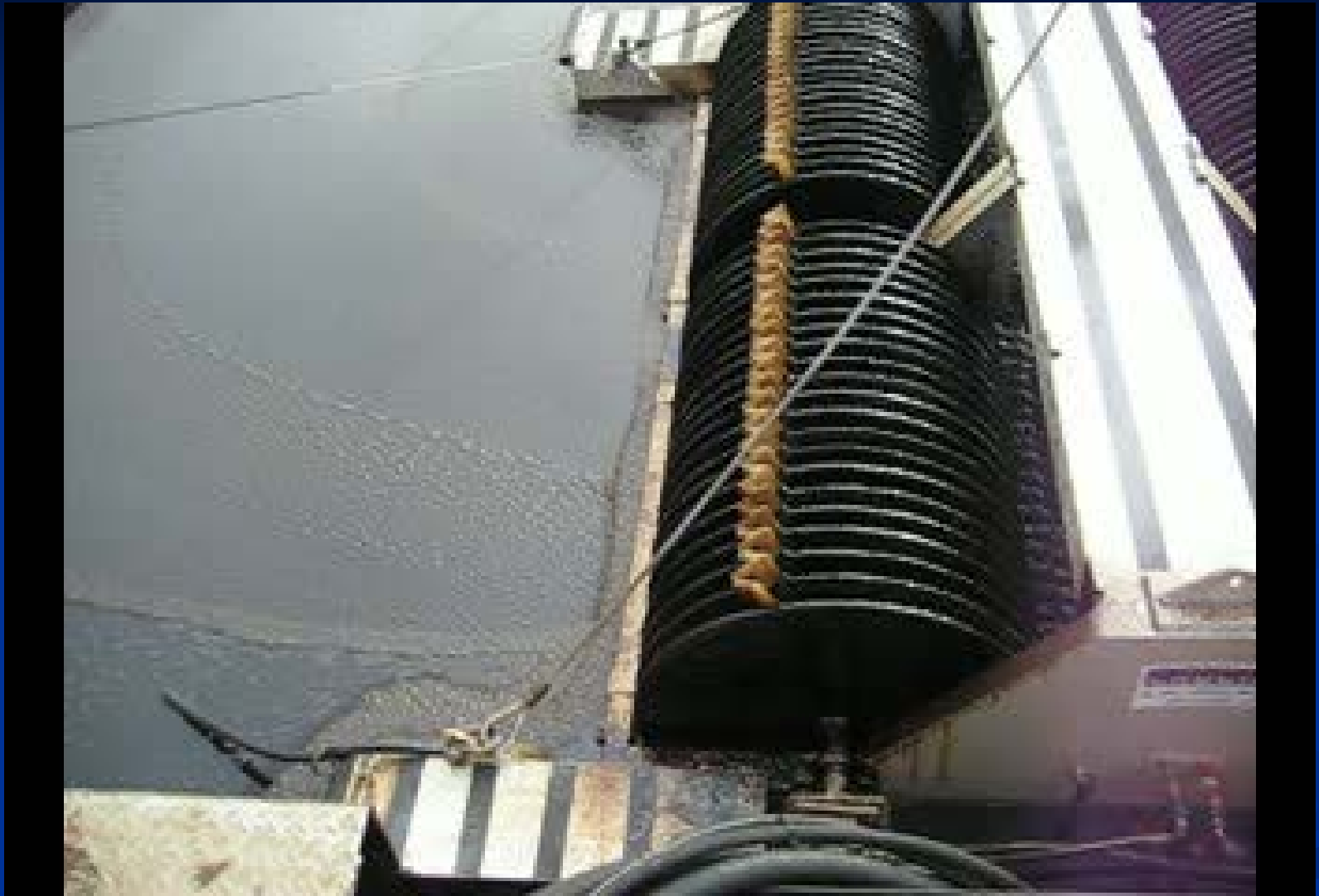
VISCOUS OIL BEING DRAWN INTO DISCS
