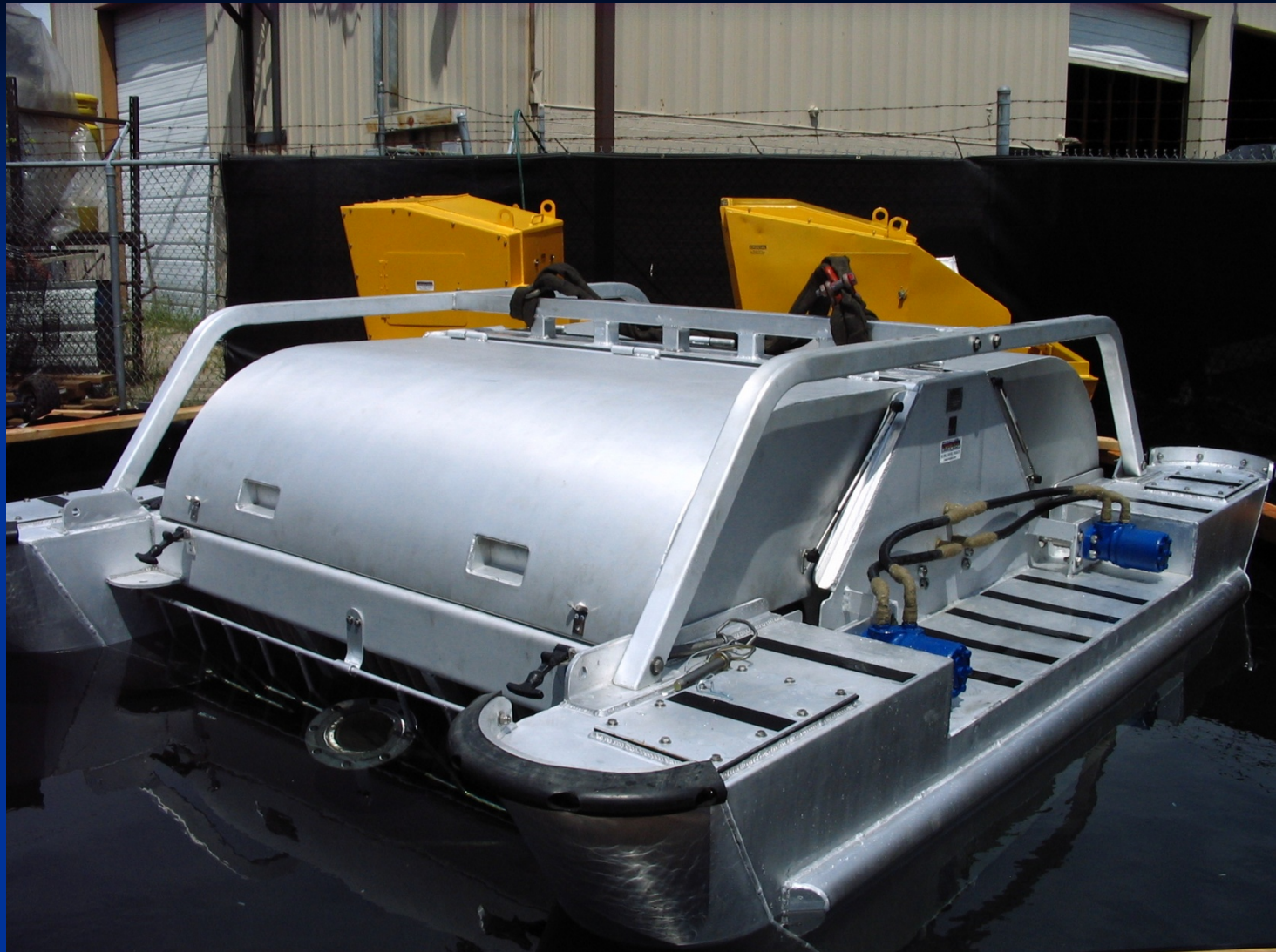
CISPRI – MODEL C-DISC 56/30 IN TEST TANK
