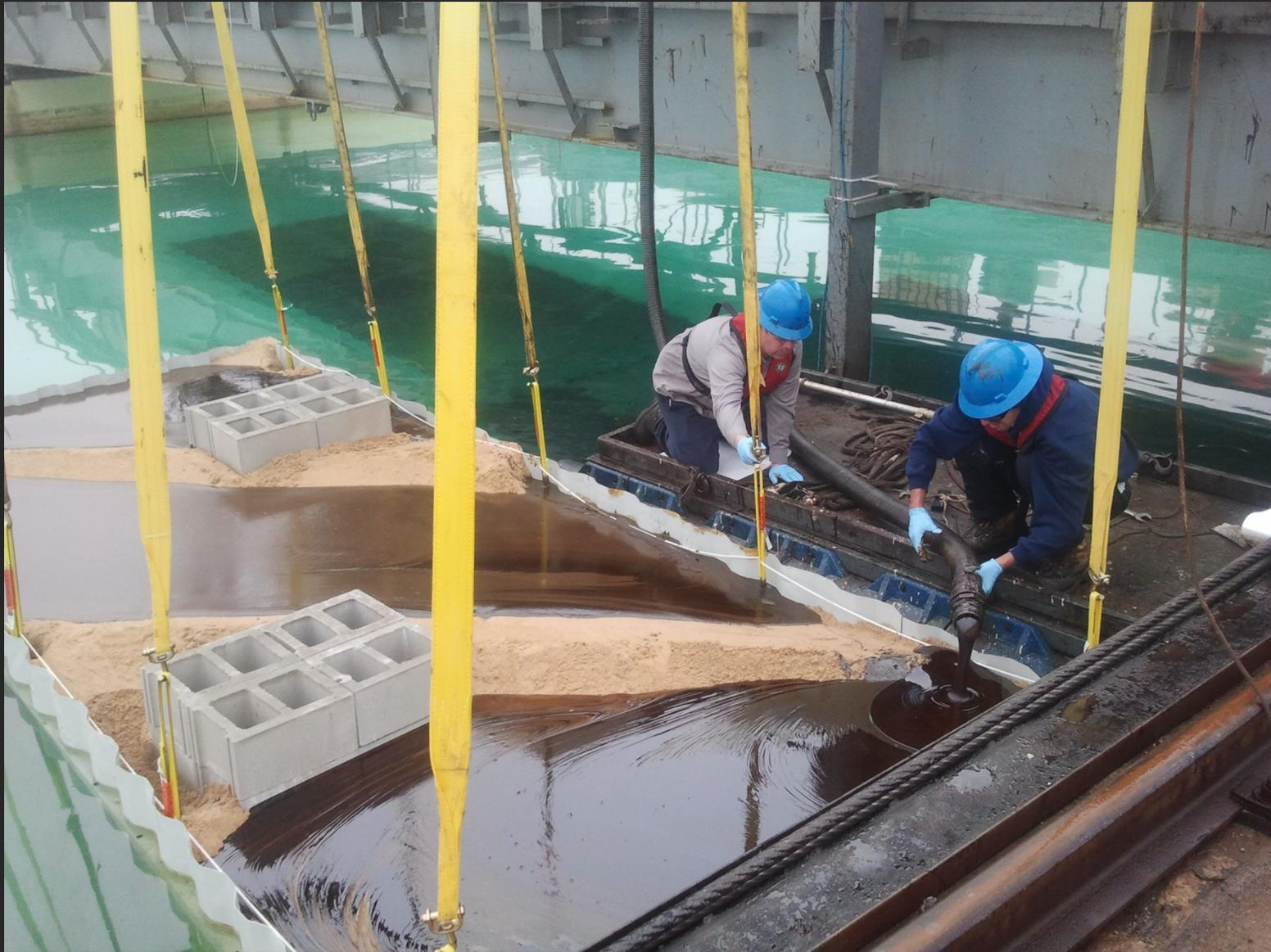
OHMSETT Tests - 150,000 Cst oil being deposited on test tray
