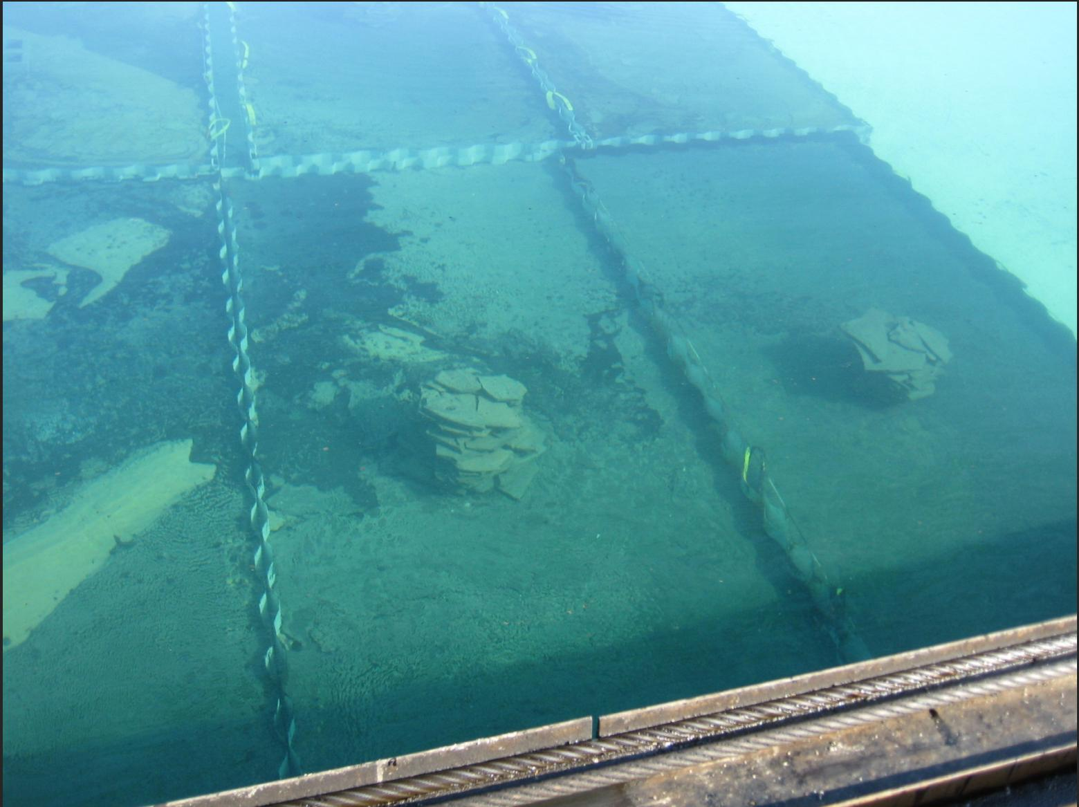
OHMSETT Tests - Trays deployed at bottom of OHMSETT tank
