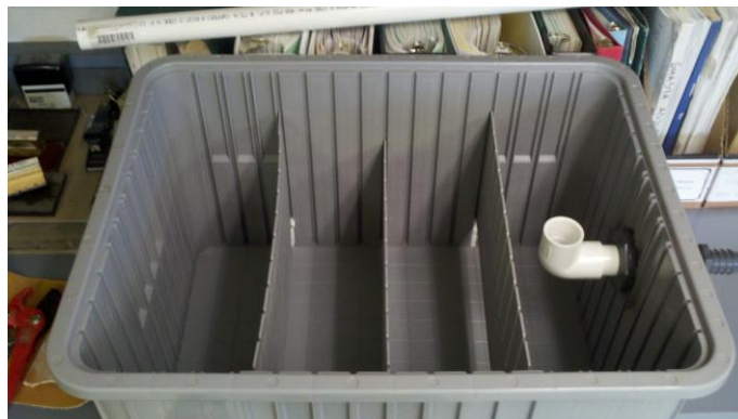
Figure 2. Interior view of biobox plates that provide suitable surfaces for mussel settlement.
