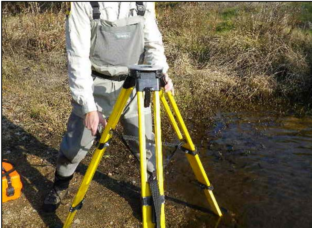
Figure 2. Example of tripod setup.
