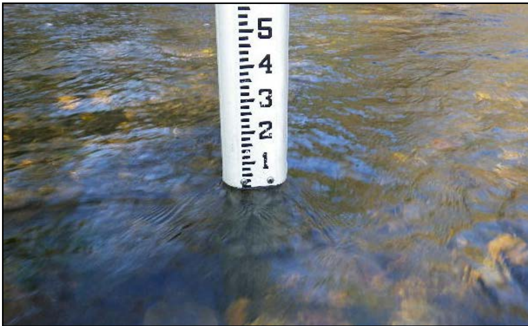
Figure 8. Example of stadia rod forming meniscus.
