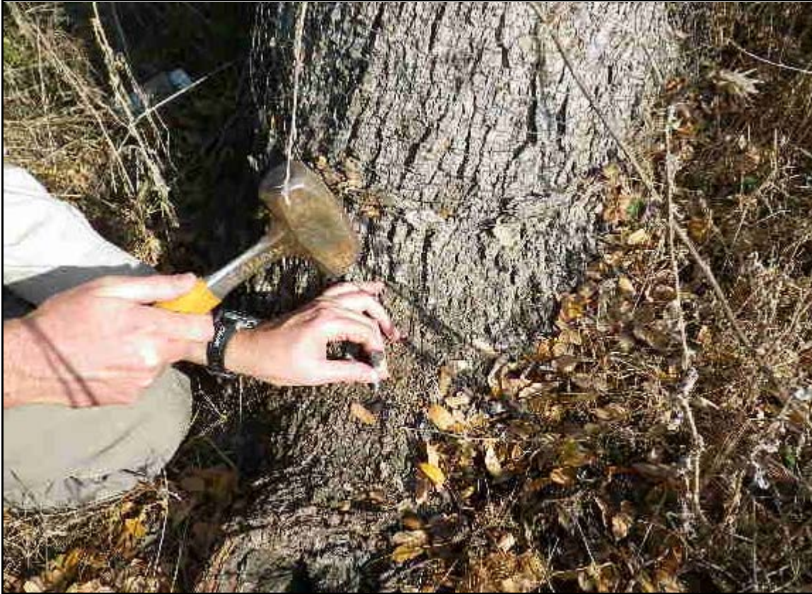
Figure 1. Example of establishing a VBM: a reference elevation for surveying using a lag bolt into a tree root.
