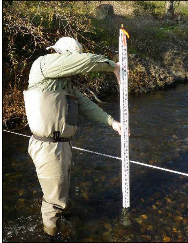
Figure 7. Example of plumb stadia rod while measuring WSEL.
