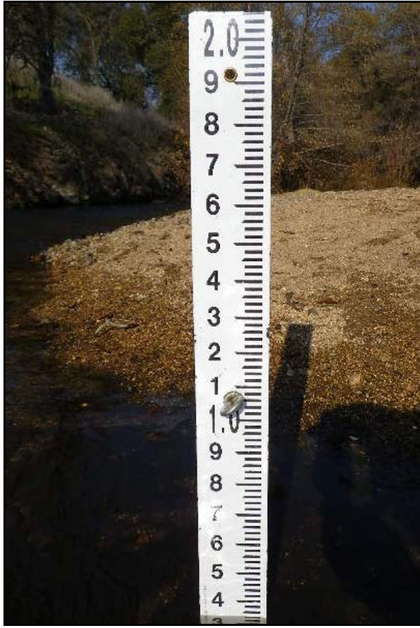
Figure 4. Example of staff gauge used to account for water surface height changes during data collection.
