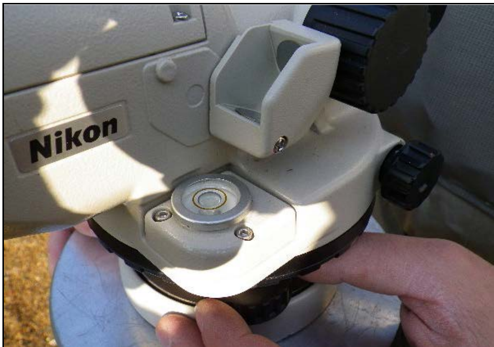
Figure 3. Example of fine adjustment dials and centered bubble on the auto level.
