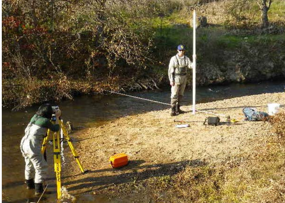
Figure 9. Example of dry bed elevation collection.
