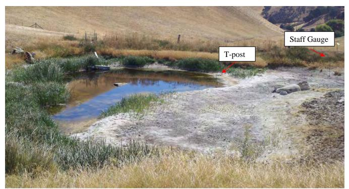
**Photograph #11.** Main Stock Pond looking southeast on September 11, 2012 showing pond draw down. The exposed t-post was an opportunity for M&A to install a second, 3 1/2-foot staff gauge in the pond. With the first rains of the 2012-2013 season, the newly installed staff gauge at this t-post was completely submerged.
