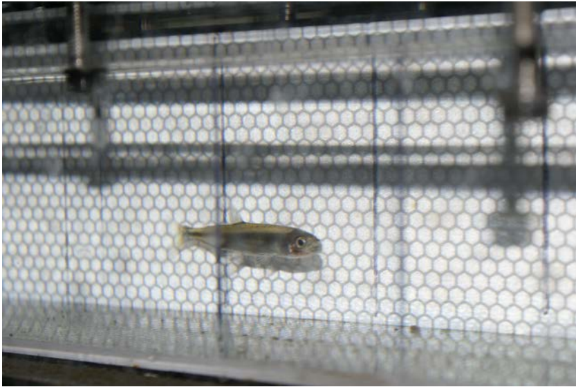
Delta smelt, swimming respirometer photo: Dennis Cocherel
