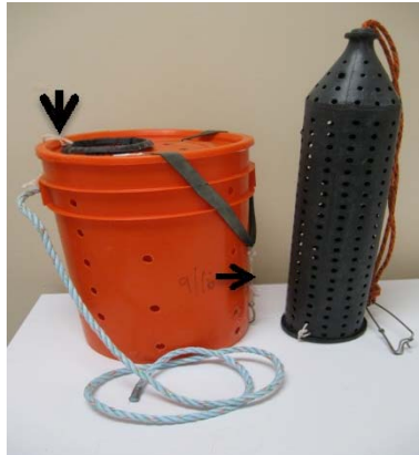
Figure 1.—Standard Korean-style trap (right) with 0.25-in. (6.4 mm) holes and a 5-gallon bucket trap (left). This is an example of one of the 0.63-in. test traps. Note the cotton twine, as indicated by the arrows, which serves as the destruct device.
