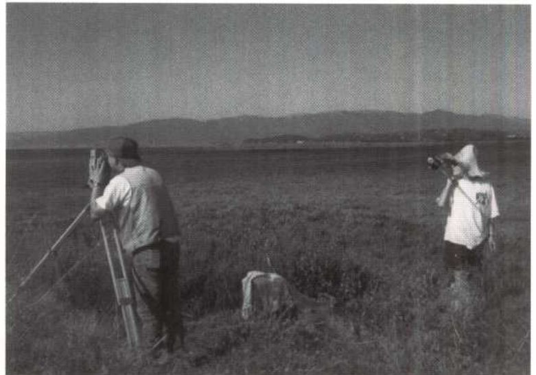
Investigating wetland restoration by surveying elevation contours (San Francisco Bay Estuary Field Station).
